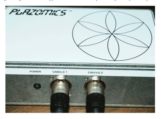
Plug the male ends of the two audio cables into the side of the PLAZOMICS unit. Make sure to push each cable in all the way until you hear a click. If you do not hear a click, the cable is not plugged in all the way.
