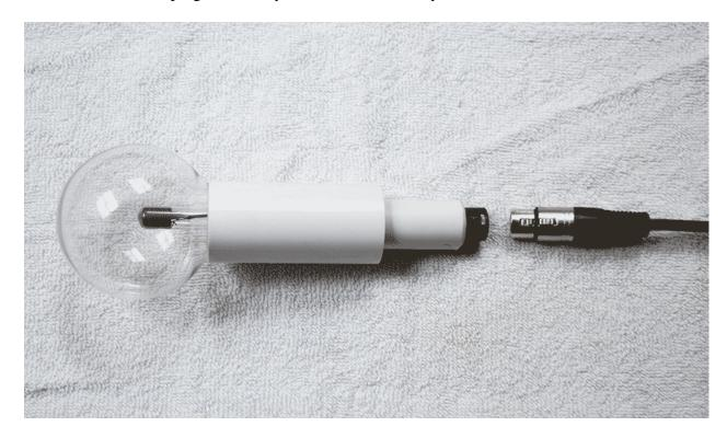
If you have the Plasma Globes, plug the female end of the audio cable into the bottom end of the globe. Push the plug all the way into the socket until you hear a click.
