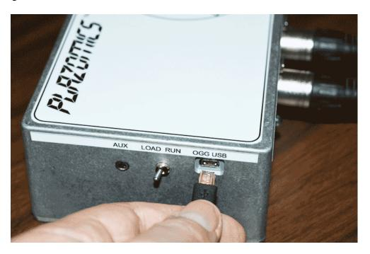
Plug the small end of the cable into the OGG USB jack on the end of the PLAZOMICS unit. Place the switch into the LOAD position.
